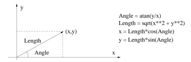
An object representing a 2D-vector will have x and y as mutable state However, we will also provide methods for Length and Angle Getting Length and Angle will compute them from x and y Setting Length or Angle will set x and y
