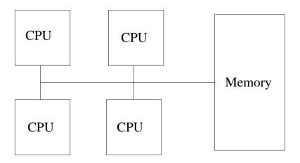
The different cores execute different pieces of code in parallel
