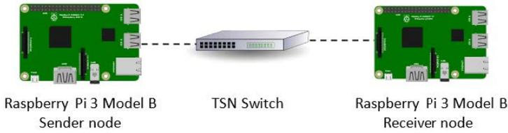
**Figure 11.2:** Heterogeneous TSN network with legacy end-stations topology.
