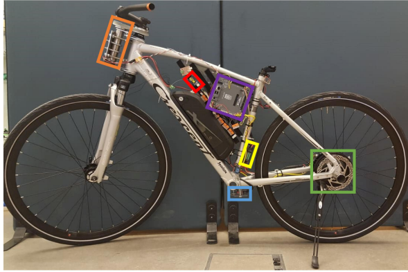
Figure 7.6: The instrumented bicycle with its rear wheel motor inside the green square. The blue box indicates the position of the VN-100, used for measuring the lean angle. Inside the yellow box is the electrical speed controller. National Instruments roboRIO is mounted on the bicycle and is highlighted by the purple box. To be able to send remote commands to the bicycle, the receiver inside the red box is utilised. The motor used to control the steering angle is highlighted by the orange rectangle.
