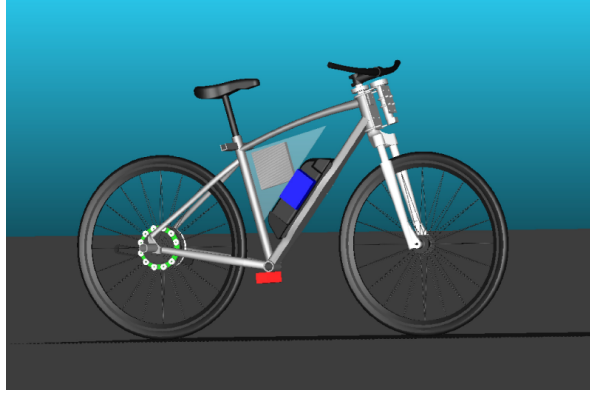
Figure 9.4: The instrumented bicycle designed in SolidWorks and imported to Adams is used as the plant in the co-simulation between Adams and Matlab.
