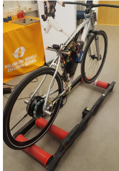
Figure 7.8: Self stabilising bicycle on a roller running with a forward speed of 14 km/h. The width of the rollers is 37 cm.
